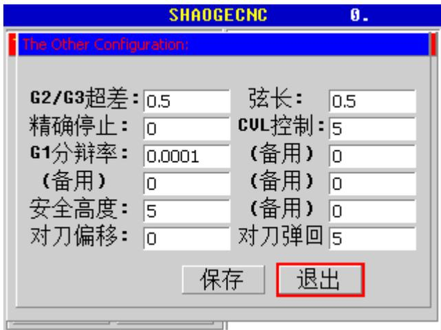
**G2/G3 超差:** Enter the G02 / G03 after manual calculations or other calculation because of accuracy issues, so that the arc center is inconsistent with the values given at the moment, there is a fault-tolerant, the system will be based on the given parameters, recalculate the optimal center coordinate
