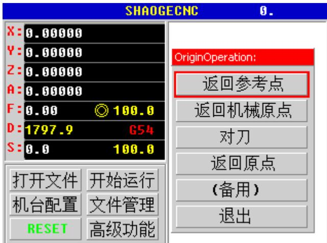
“返回参考点” Z-axis height to rise to safety, all other axes back to the specified location, Z axis return to the specified location (in the mechanical origin can be set at this point)
