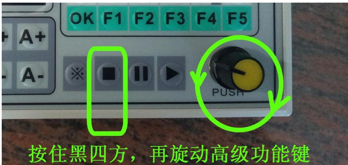
In standby (not running processing) for speed: Press and hold the stop button (黑四方键), while another swirling advanced function keys, you can directly adjust the speed percentage, on the main screen you can see the speed percentage (I: 100-1) display.
